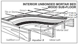
LIMITATIONS: Aquabar "B" hardwood floor and tile underlayment is not a vapor barrier or a waterproof membrane and should not be used in waterproofing assemblies where a moisture or vapor barrier is specified. Do not leave exposed to direct moisture contact or use in areas that are soaked or saturated for extended periods of time, such as gang showers, saunas, steam rooms, pools, hot tubs and exterior areas.
